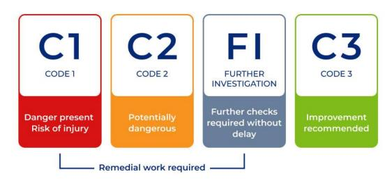
• Code 3 (C3) is described as 'Improvement recommended.' A code C3 is to be used to indicate that certain items have been identified as not complying with the requirements of the current issue of BS 7671, but that the users of the installation are not in any immediate or potential danger as a result. Careful consideration should be given to the safety benefits of improving those aspects of the installation. A code C3, in itself, should not warrant an overall unsatisfactory report.
